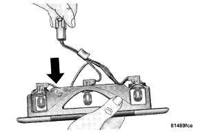
4. Turn desired bulb socket 1/4-turn and remove socket and bulb from housing.
